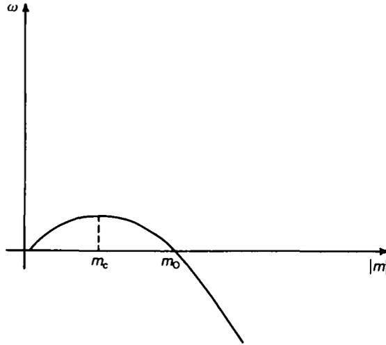
FIG. 1. Dependence of the stability eigenvalue  $\omega$  on wavenumber  $m$  for small perturbations from the planar dissolution interface.
