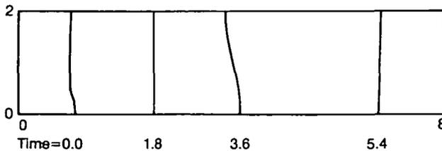
FIG. 3. Temporal sequence of porosity contours for a stable system. The parameter values used are:  $\varphi_0 = 0.1$ ,  $\varphi_f = 0.2$ ,  $c^{ca}/\rho = 0.05$ ,  $p_f' = -1$ . The figure shows porosity contours with  $\varphi = 0.15$ .
