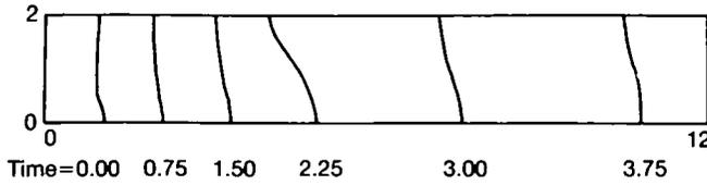
FIG. 4. Temporal sequence of porosity contours with  $\varphi = 0.15$  for an unstable system. The parameter values used here are the same as those in Fig. 3 except that  $p'_i = -2$ .
