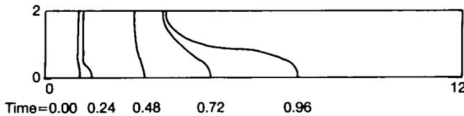
FIG. 5. Temporal sequence of porosity contours with  $\varphi = 0.15$  for a highly unstable system. Same parameter values as in Fig. 3 are used here except that now for  $p'_i = -10$ .
