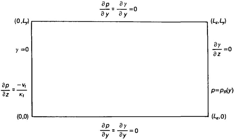
FIG. 2. Domain in which numerical simulation of the reactive percolation equations is carried out. Note that in view of the reflection symmetry about the  $y = 0$  axis, the numerical solutions should be interpreted in a domain twice as large in the  $y$ -direction, the physical domain being  $-L_y \leq y \leq +L_y$ .
